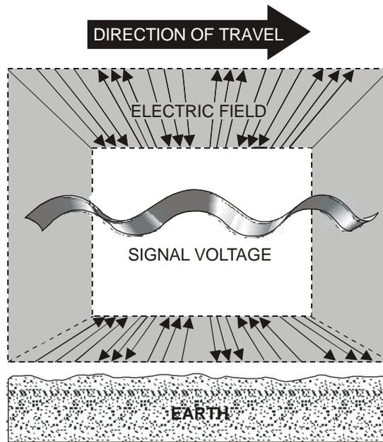
Figure 2-4. Horizontal Polarization.
