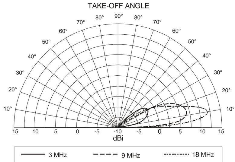
Figure 4-32. 50-Foot Vertical Half-Rhombic (Vertical Pattern), 1,000 Feet Long.
