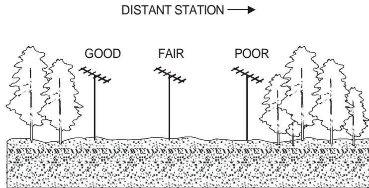
Figure 8-4. Directional Antennas Sited in a Clearing.
