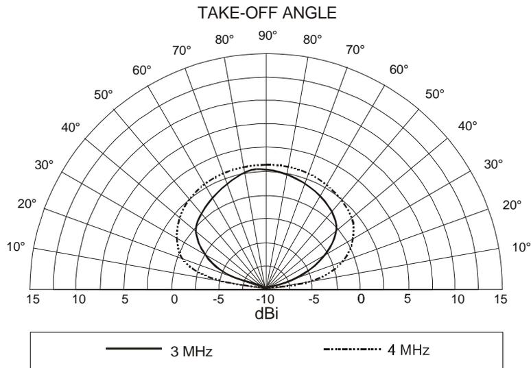
**Figure 4-19. 40-Foot Inverted L (Vertical Pattern),
