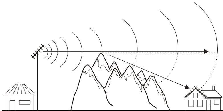
Figure 1-7. Diffracted Wave.
