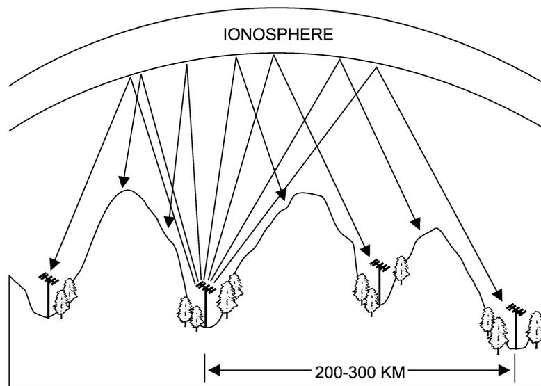
Figure 4-33. NVIS Propagation.
