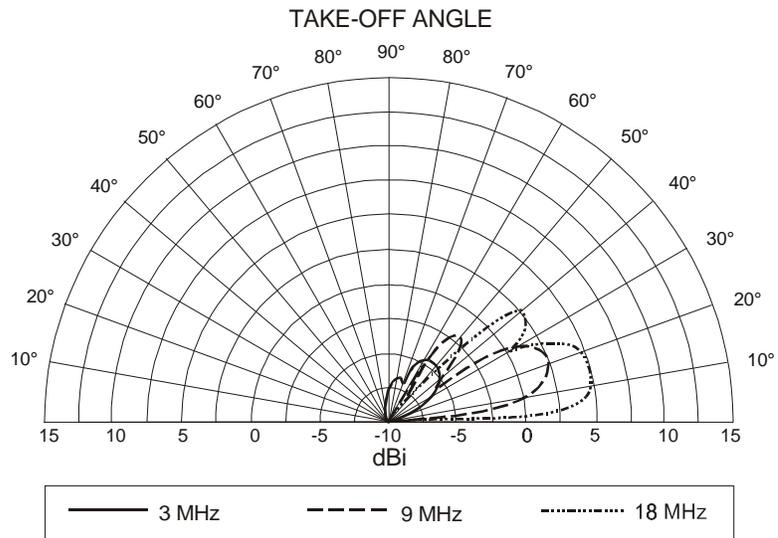
Figure 4-31. 50-Foot Vertical Half-Rhombic (Vertical Pattern), 500 Feet Long.
