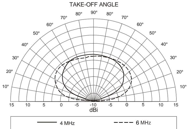
**Figure 4-21. 40-Foot Inverted L (Vertical Pattern),
