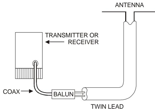
Figure 3-3. Balun Placed at the Transmitter or Receiver.
