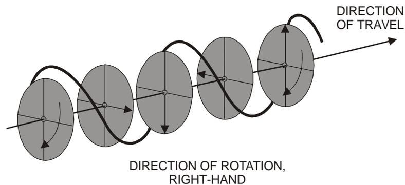
**Figure 2-5. Circular Polarization.**
