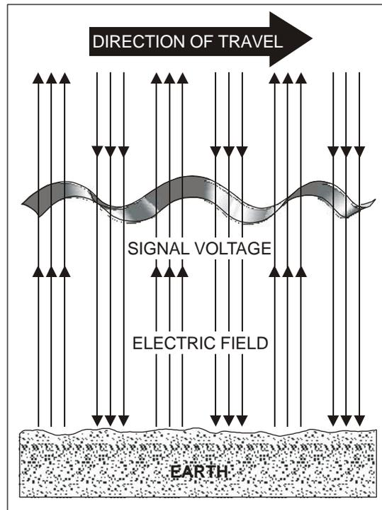
Figure 2-3. Vertical Polarization.
